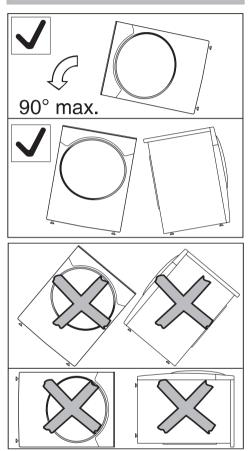
⚠ If the tumble dryer has not been transported as described, then it must be left to stand for at least 1 hour <u>before</u> it is connected to the electricity supply. Otherwise the heat pump can be damaged.
